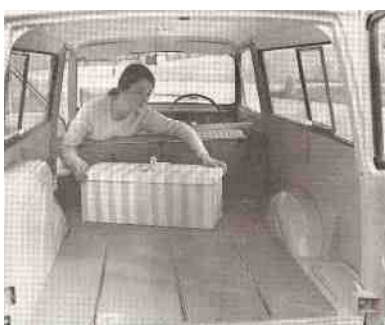
The comfortable rear seat folds flat into the floor, giving a full-size loading area with accommodation for driver and one passenger.
